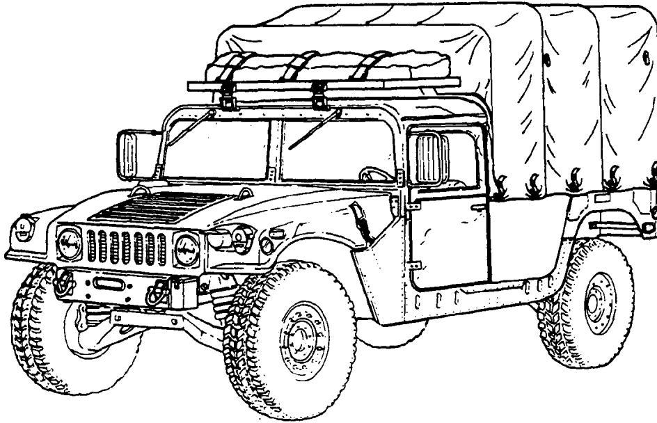
M1097/M1097A1/M1097A2/M1123 (WITH L119 KIT INSTALLED) (WITHOUT WINCH, TOWED VULCAN SYSTEMS (TVS) MOVER)
